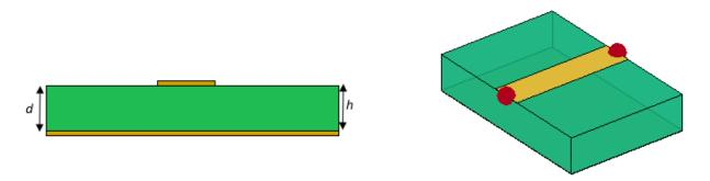
When the pcbComponent has a single dielectric layer, the BoardThickness (h) should be equal to dielectric thickness (d). If h is not equal to d, then d is updated to match h.
