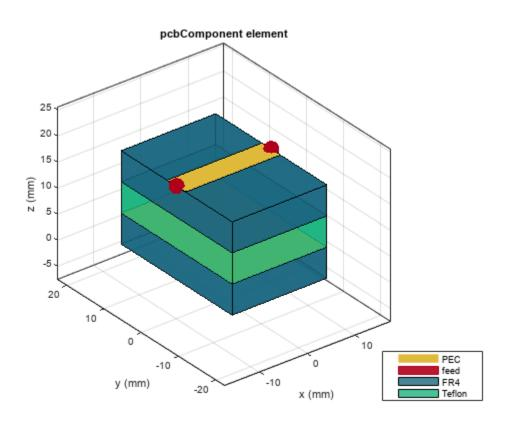
In this use case, there is a dielectric layer present above the top metal layer and air dielectric separates the top and bottom metal layers. Add another dielectric layer below the bottom metal layer. The dielectric layer which is present above the top metal layer is considered as coating and is included in the BoardThickness calculation. The BoardThickness (h) will be the sum of dielectric layers below the top metal layer (*ie.* h = d2 + d3).
