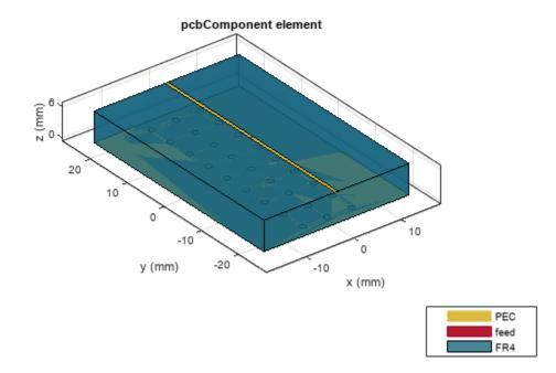
Modify the above use case by removing the top and bottom air dielectric layers as show in figure. This use case is now a single-layer dielectric pcbComponent. Now you can change the dielectric thickness by changing the BoardThickess.(h = d).
