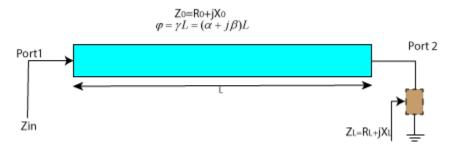
The complex propagation constant for this line is given by the equation:
