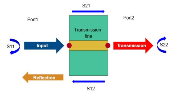
$S_{21}$  is the measure of the transmitted signal from port 2 relative to the input entering port 1.  $S_{11}$  is the measure of the reflected signal from port 1 relative to the input entering port 1.
